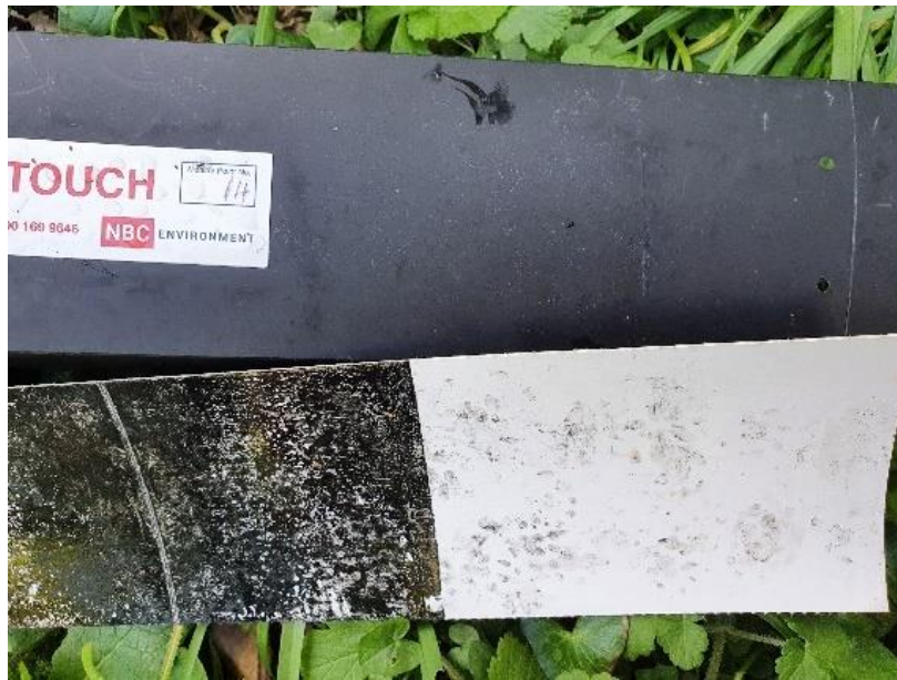
Figure 3: Tracking tunnel and ink plate.
